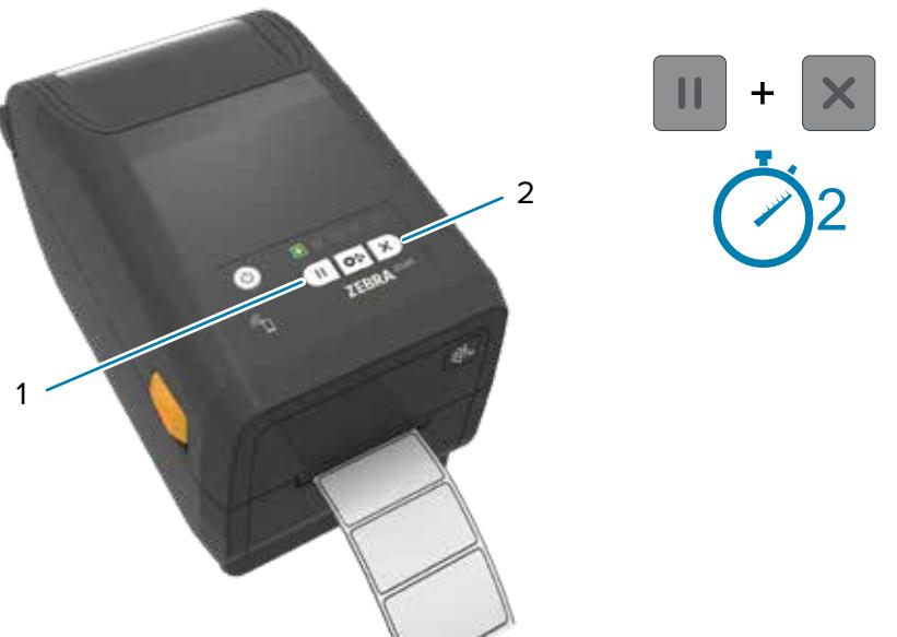
Press and hold the Pause (1) and Cancel (2) buttons for two seconds to line up the labels.
