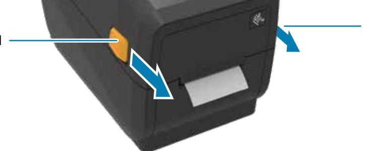
Slide the release latches (1) to the front to unlock the cover.
