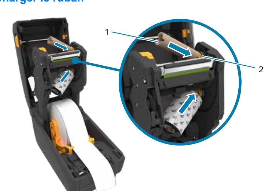
Push the right side of the spool (1) onto the spring-loaded spindle (2).
