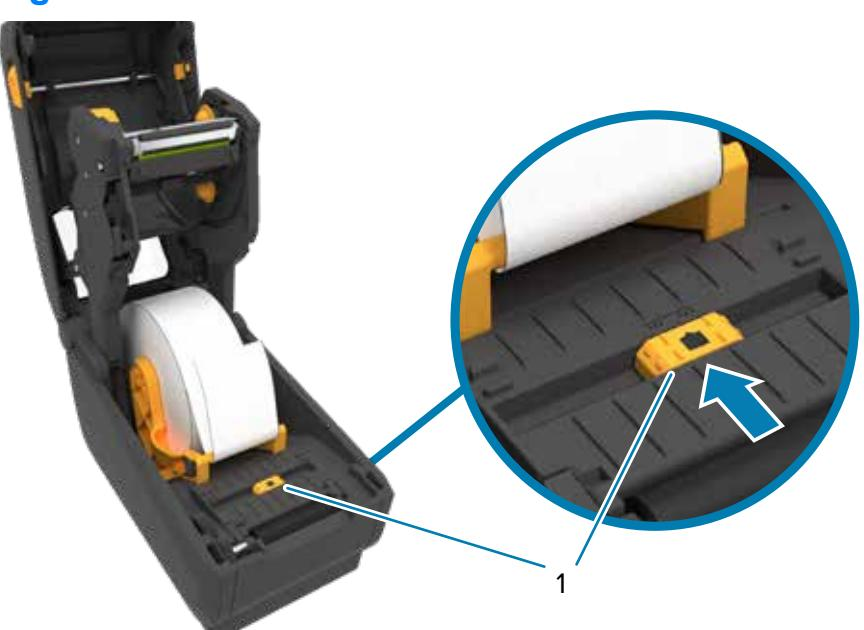
Align the sensor (1) to the center of the roll for regular labels and receipts.
