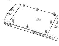
Follow the same steps to remove or install the extended battery and extended battery cover.
