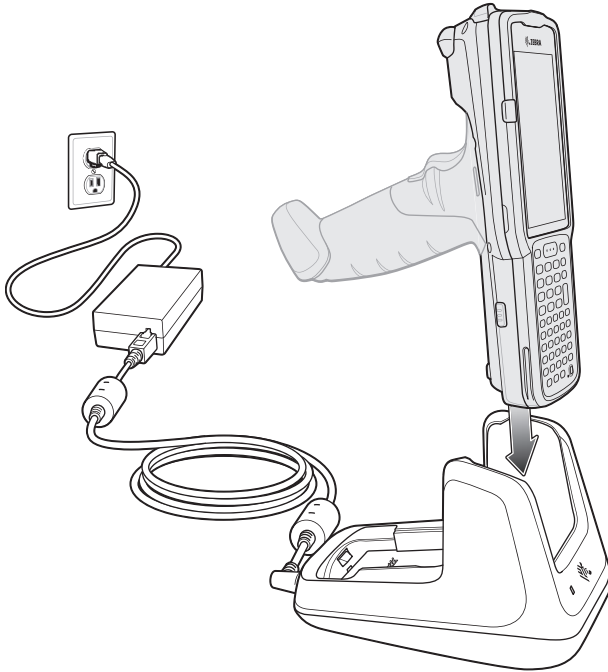
Figure 13 MC33XX Battery Charging
